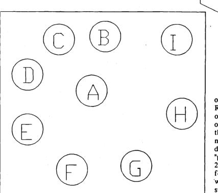
of 3" long, 5/8" diameter "pegs". Reduce the diameter on one end of each peg for approximately 1" of length so that the pegs fit in the holes without binding. You now have a bending fork with 36 different spans between the "pegs", running from 0.26 to 2.87 inches (see the table below for the combination of holes which gives each span). If the stock that you're bending is too heavy for this jig, just scale up to 3/4" or 1" pegs. When using
